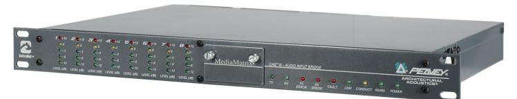
The CAB<sup>-</sup> 8i is an eight-channel, input only, digitally controlled preamp using 24-bit analog-to-digital converters. Includes mic preamps with software-controllable 48V phantom power, mic/line selection and analog gain.
